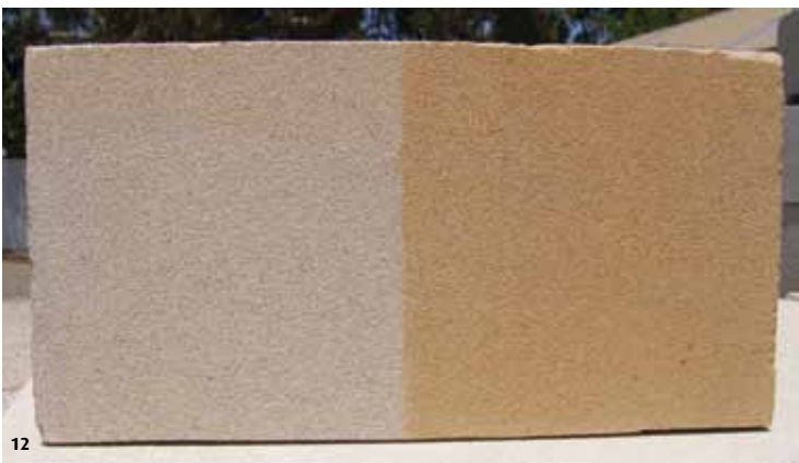
Photo 11: The new spires of St Mary's Cathedral, Sydney – Wondabyne stone. Photo 12: A piece of McCaffrey's stone artificially and permanently coloured. (Photos: Jasper Swann, 2007)
