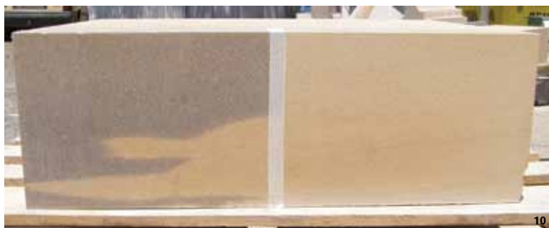
Photo 7: Guinea Gold stone used for the new portico at Sydney Grammar School. Photo 8: A piece of McCaffrey’s (top) above a piece of Guinea Gold, eight weeks after sawing. Photo 9: Irregular manganese staining on a piece of Guinea Gold and ( photo 10 ) its removal using a weak hydrochloric acid solution. (Photos: Jasper Swann, 2007)
